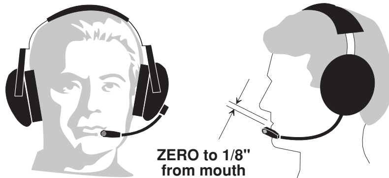
Figure 12 - Correct Positioning of Boom and Microphone
